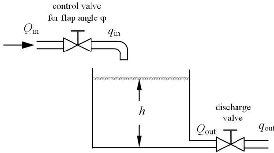
Fig. 7. A nonlinear liquid-level system
