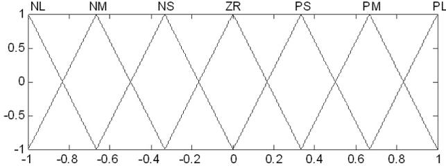
Fig. 4. The membership functions of  $e$ ,  $\dot{e}$  and  $u$ .
