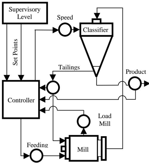
Figure 1. Block diagram of the cement milling circuit
